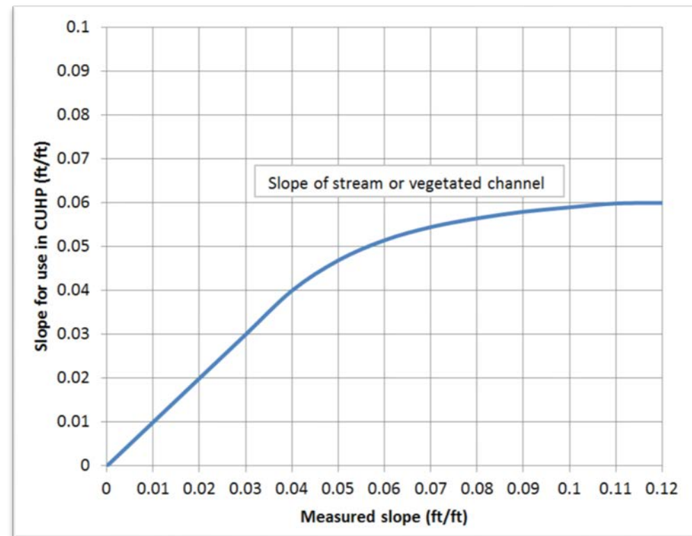
Figure 3-2: Slope correction for streams and vegetated channels USDCM Figure 6-4 (Reference 1)
